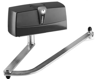
Irreversible geared motor suitable for gates installed on large columns, available in 230 Vac and 24 Vdc versions. Built-in electromechanical open and close limit switches, with sturdy articulated anti-shearing arm in galvanised steel.
