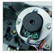
**OPTICAL ENCODER** Obstacle detection and anticrushing safety ensured by the optical encoder. The encoder also manages the deceleration in the closing and opening phases and the adjustment of the gate stroke which doesn't require a limit switch.
