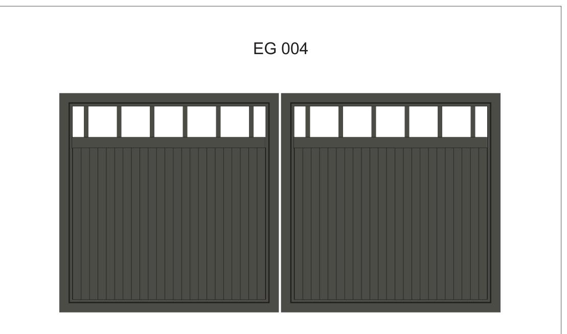
MAIN FRAME - Easy gate main frame 92x48x3. Mitred corners with welded 3mm thick corner braces giving 6mm wall thickness at each corner. INFILL - 38x16 vertical slats at nominal 100mm spacing (adjust to suit your requirements). Bottom slats 65x16 horizontal and no spacing. FINISH - Pre treatment and powder coat. Kit includes covers to conceal all infill fastening points. SIZE RESTRICTIONS - Sliding maximum width 6450mm. Swing maximum width 3200mm.
