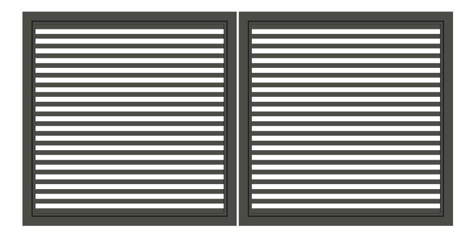
MAIN FRAME - Easy gate main frame 92x48x3. Mitred corners with welded 3mm thick corner braces giving 6mm wall thickness at each corner. INFILL - 38x16 horizontal slats at nominal 45mm spacing (adjust to suit your requirements). FINISH - Pre treatment and powder coat. Kit includes covers to conceal all infill fastening points. SIZE RESTRICTIONS - Sliding maximum width 6450mm. Swing maximum width 3200mm.
