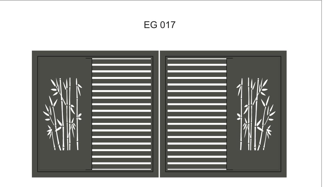
MAIN FRAME - Easy gate main frame 92x48x3. Mitred corners with welded 3mm thick corner braces giving 6mm wall thickness at each corner. INFILL - 65x16 horizontal slats at nominal 15mm spacing (adjust to suit your requirements). Decorative panel can be adjusted to anywhere in the gate. FINISH - Pre treatment and powder coat. Kit includes covers to conceal all infill fastening points. SIZE RESTRICTIONS - Sliding maximum width 6450mm. Swing maximum width 3200mm.
