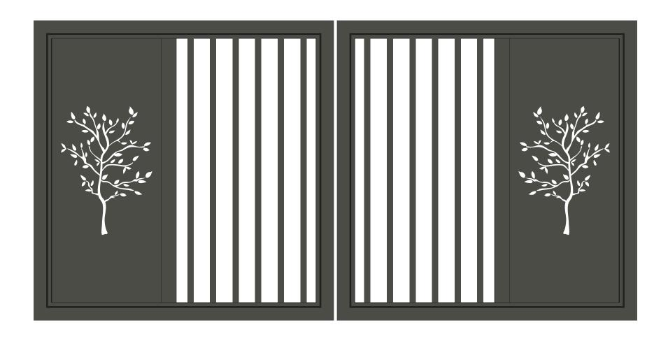
MAIN FRAME - Easy gate main frame 92x48x3. Mitred corners with welded 3mm thick corner braces giving 6mm wall thickness at each corner. INFILL - 38x16 vertical slats at nominal 100mm spacing (adjust to suit your requirements). Decorative panel can be adjusted to anywhere in the gate. FINISH - Pre treatment and powder coat. Kit includes covers to conceal all infill fastening points. SIZE RESTRICTIONS - Sliding maximum width 6450mm. Swing maximum width 3200mm.
