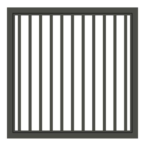
MAIN FRAME - Standard gate main frame 75x50x3. Mitred corners with extruded 5mm thick corner stakes. INFILL - 38x16 vertical slats at nominal 100mm spacing (adjust to suit your requirements). FINISH - Pre treatment and powder coat. Kit includes covers to conceal all infill fastening points. SIZE RESTRICTIONS - Maximum width 1500mm. Larger gates use Easy gate frame and corners.
