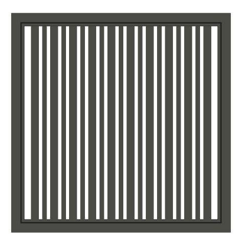
MAIN FRAME - Standard gate main frame 75x50x3. Mitred corners with extruded 5mm thick corner stakes. INFILL - Alternate 65x16 and 38x16 vertical slats at nominal 15mm spacing (adjust to suit your requirements). FINISH - Pre treatment and powder coat. Kit includes covers to conceal all infill fastening points. SIZE RESTRICTIONS - Maximum width 1500mm. Larger gates use Easy gate frame and corners.
