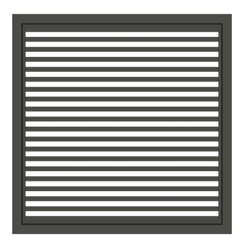
MAIN FRAME - Standard gate main frame 75x50x3. Mitred corners with extruded 5mm thick corner stakes. INFILL - 38x16 horizontal slats at nominal 45mm spacing (adjust to suit your requirements). FINISH - Pre treatment and powder coat. Kit includes covers to conceal all infill fastening points. SIZE RESTRICTIONS - Maximum width 1500mm. Larger gates use Easy gate frame and corners.
