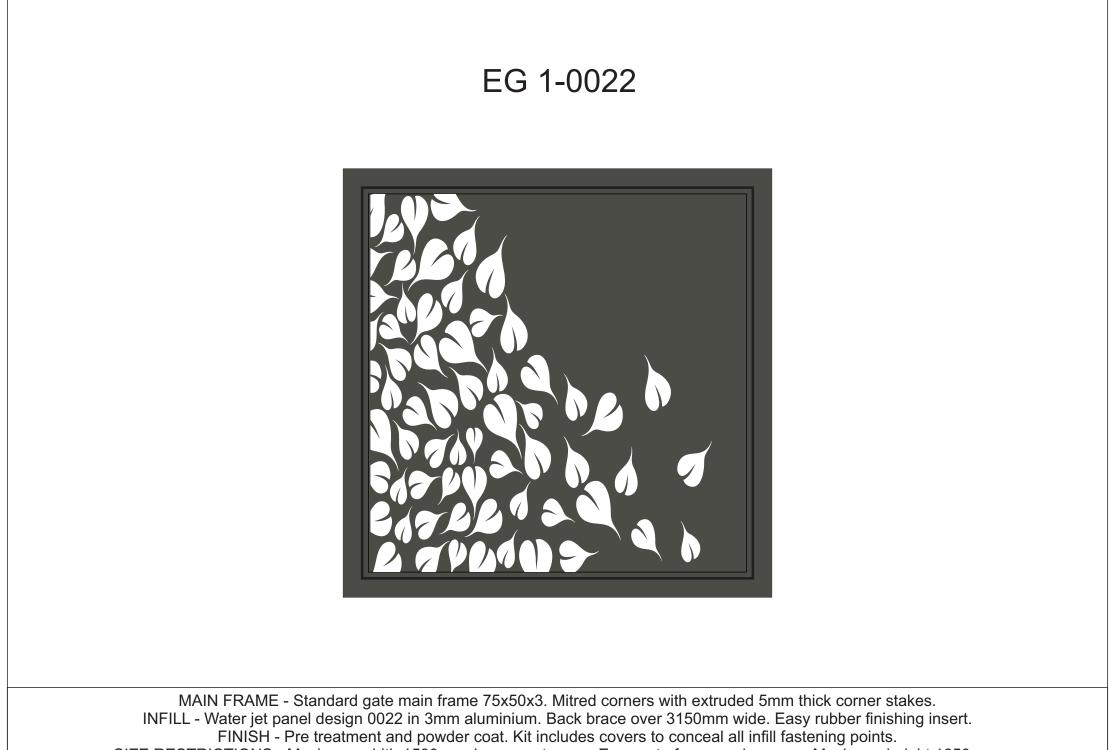
SIZE RESTRICTIONS - Maximum width 1500mm. Larger gates use Easy gate frame and corners. Maximum height 1650mm.
