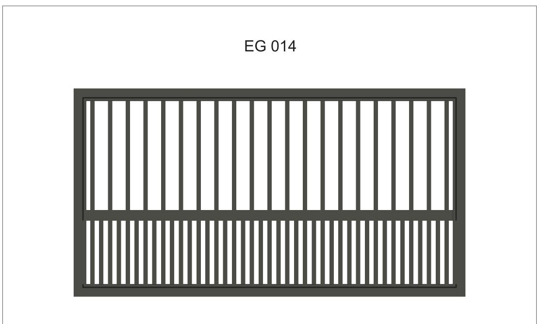
MAIN FRAME - Easy gate main frame 92x48x3. Mitred corners with welded 3mm thick corner braces giving 6mm wall thickness at each corner. INFILL - 38x16 vertical slats at nominal 100mm spacing (adjust to suit your requirements). Bottom slats half top spacing. FINISH - Pre treatment and powder coat. Kit includes covers to conceal all infill fastening points. SIZE RESTRICTIONS - Sliding maximum width 6450mm. Swing maximum width 3200mm.
