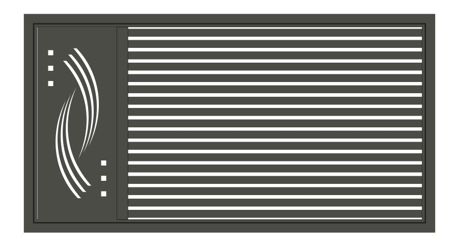
MAIN FRAME - Easy gate main frame 92x48x3. Mitred corners with welded 3mm thick corner braces giving 6mm wall thickness at each corner. INFILL - 65x16 horizontal slats at nominal 15mm spacing (adjust to suit your requirements). Decorative panel can be adjusted to anywhere in the gate. FINISH - Pre treatment and powder coat. Kit includes covers to conceal all infill fastening points. SIZE RESTRICTIONS - Sliding maximum width 6450mm. Swing maximum width 3200mm.
