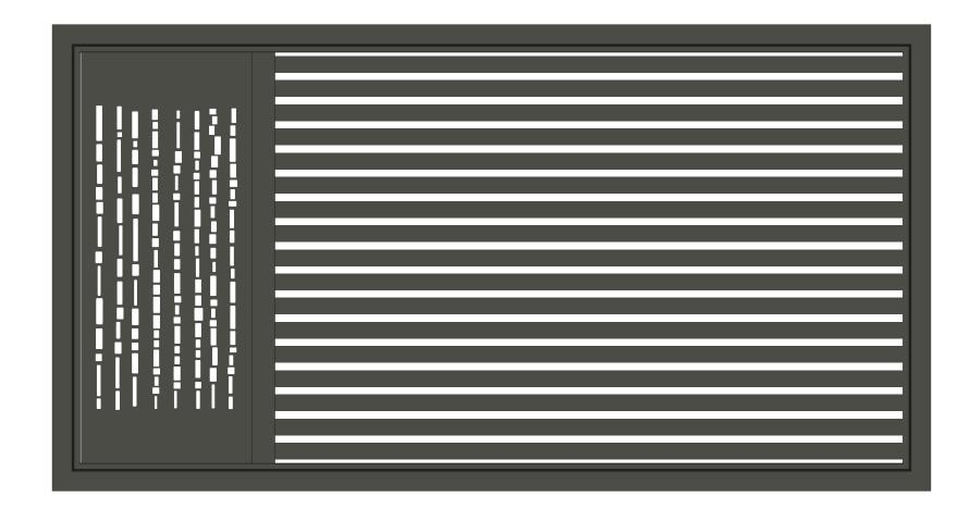
MAIN FRAME - Easy gate main frame 92x48x3. Mitred corners with welded 3mm thick corner braces giving 6mm wall thickness at each corner. INFILL - 65x16 horizontal slats at nominal 15mm spacing (adjust to suit your requirements). Decorative panel can be adjusted to anywhere in the gate. FINISH - Pre treatment and powder coat. Kit includes covers to conceal all infill fastening points. SIZE RESTRICTIONS - Sliding maximum width 6450mm. Swing maximum width 3200mm.
