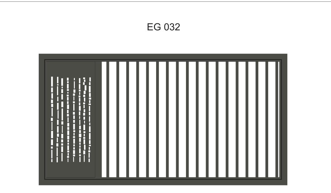
MAIN FRAME - Easy gate main frame 92x48x3. Mitred corners with welded 3mm thick corner braces giving 6mm wall thickness at each corner. INFILL - 38x16 vertical slats at nominal 100mm spacing (adjust to suit your requirements). Decorative panel can be adjusted to anywhere in the gate. FINISH - Pre treatment and powder coat. Kit includes covers to conceal all infill fastening points. SIZE RESTRICTIONS - Sliding maximum width 6450mm. Swing maximum width 3200mm.
