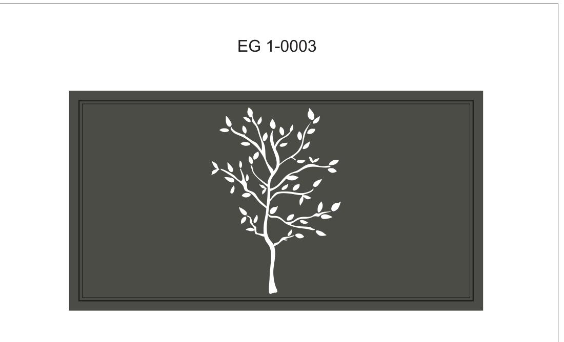
MAIN FRAME - Easy gate main frame 92x48x3. Mitred corners with welded 3mm thick corner braces giving 6mm wall thickness at each corner. INFILL - Water jet panel design 0003 in 3mm aluminium. Back brace over 3150mm wide. Easy rubber finishing insert. FINISH - Pre treatment and powder coat. Kit includes covers to conceal all infill fastening points. SIZE RESTRICTIONS - Sliding maximum width 6450mm. Swing maximum width 3200mm. Maximum height 1650mm.
