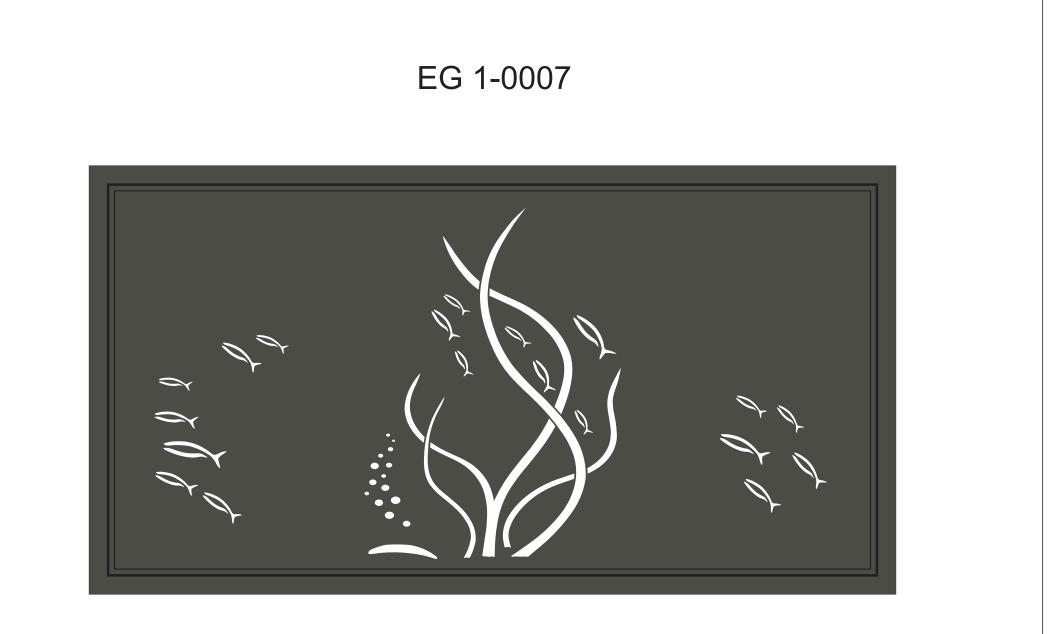
MAIN FRAME - Easy gate main frame 92x48x3. Mitred corners with welded 3mm thick corner braces giving 6mm wall thickness at each corner. INFILL - Water jet panel design 0007 in 3mm aluminium. Back brace over 3150mm wide. Easy rubber finishing insert. FINISH - Pre treatment and powder coat. Kit includes covers to conceal all infill fastening points. SIZE RESTRICTIONS - Sliding maximum width 6450mm. Swing maximum width 3200mm. Maximum height 1650mm.
