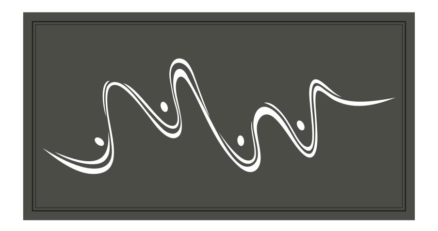
MAIN FRAME - Easy gate main frame 92x48x3. Mitred corners with welded 3mm thick corner braces giving 6mm wall thickness at each corner. INFILL - Water jet panel design 0019 in 3mm aluminium. Back brace over 3150mm wide. Easy rubber finishing insert. FINISH - Pre treatment and powder coat. Kit includes covers to conceal all infill fastening points. SIZE RESTRICTIONS - Sliding maximum width 6450mm. Swing maximum width 3200mm. Maximum height 1650mm.
