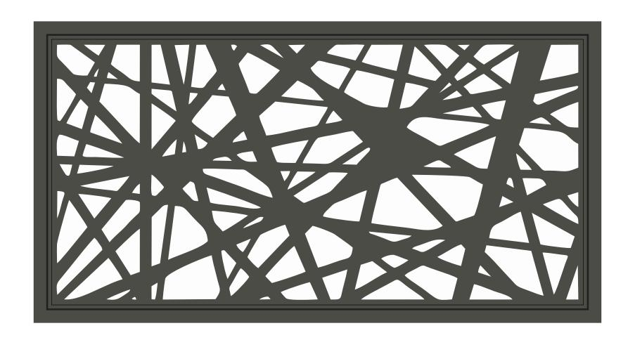
MAIN FRAME - Easy gate main frame 92x48x3. Mitred corners with welded 3mm thick corner braces giving 6mm wall thickness at each corner. INFILL - Water jet panel design 0062 in 3mm aluminium. Back brace over 3150mm wide. Easy rubber finishing insert. FINISH - Pre treatment and powder coat. Kit includes covers to conceal all infill fastening points. SIZE RESTRICTIONS - Sliding maximum width 6450mm. Swing maximum width 3200mm. Maximum height 1650mm.
