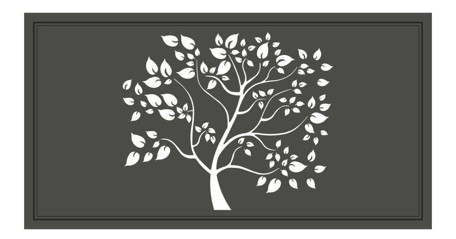
MAIN FRAME - Easy gate main frame 92x48x3. Mitred corners with welded 3mm thick corner braces giving 6mm wall thickness at each corner. INFILL - Water jet panel design 0064 in 3mm aluminium. Back brace over 3150mm wide. Easy rubber finishing insert. FINISH - Pre treatment and powder coat. Kit includes covers to conceal all infill fastening points. SIZE RESTRICTIONS - Sliding maximum width 6450mm. Swing maximum width 3200mm. Maximum height 1650mm.
