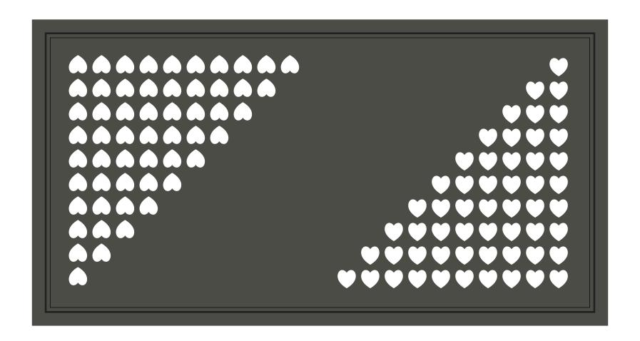
MAIN FRAME - Easy gate main frame 92x48x3. Mitred corners with welded 3mm thick corner braces giving 6mm wall thickness at each corner. INFILL - Water jet panel design 0079 in 3mm aluminium. Back brace over 3150mm wide. Easy rubber finishing insert.
