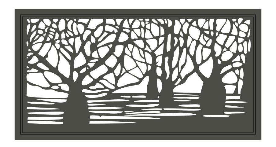
MAIN FRAME - Easy gate main frame 92x48x3. Mitred corners with welded 3mm thick corner braces giving 6mm wall thickness at each corner. INFILL - Water jet panel design 0092 in 3mm aluminium. Back brace over 3150mm wide. Easy rubber finishing insert. FINISH - Pre treatment and powder coat. Kit includes covers to conceal all infill fastening points. SIZE RESTRICTIONS - Sliding maximum width 6450mm. Swing maximum width 3200mm. Maximum height 1650mm.
